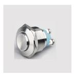
Diameter: Ø 22mm Switch Rating: 5A/250VAC Contact Configuration: 1NO Operation Type: Momentary The Front Shape: High The Crust Material: Stainless steel
