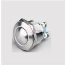
Diameter: Ø 22mm Switch Rating: 5A/250VAC Contact Configuration: 1NO Operation Type: Momentary The Front Shape: Flat The Crust Material: Stainless steel
